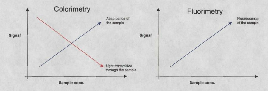
Colorimetry is used to measure NO3/NO2, PO4 and SiO4. The attenuation of a beam of light is recorded. The light passing through the sample decreases with increasing concentration. This is shown by the red line. Absorbance increases linearly (to a point) with concentration as shown by the blue line. This is in accordance with the Beer-Lambert Law.
